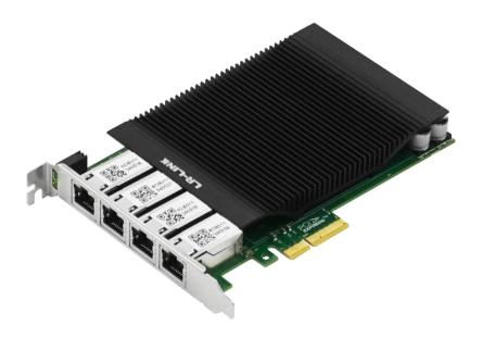
LRES2004PT-POE is a quad-port copper gigabit ethernet PCI Express x4 PoE+ ethernet frame grabber independently developed by Shenzhen Lianrui Electronics Co., Ltd. based on the Intel I350 chip. It is also compatible with PCIe x8 and x16. The grabber adapter design is mainly designed for industrial field visual inspection servers and equipment, visual field clients, fast mobile ethernet data transmission equipment, etc., and is also suitable for ordinary servers.
